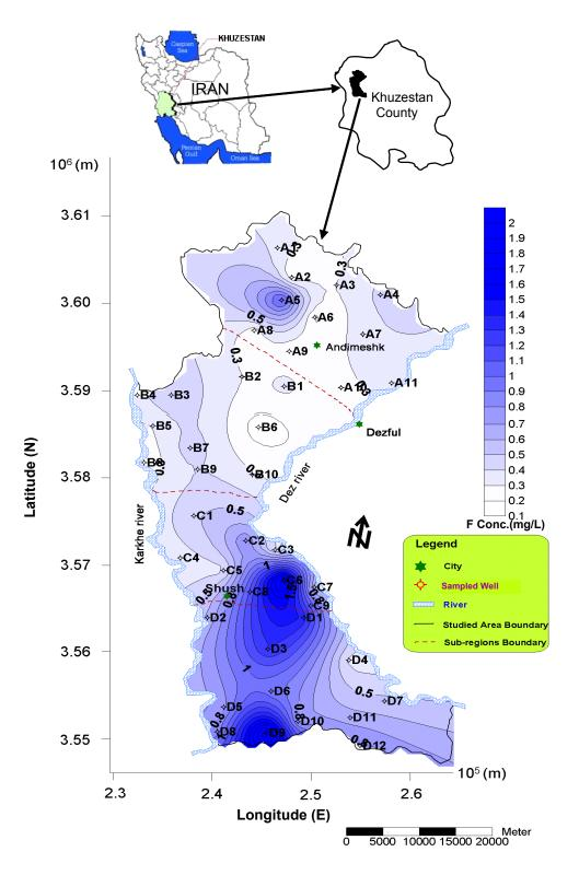
Figure 1. Distribution of F concentration in the Shush aquifer (mg/L).
