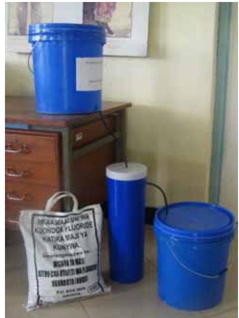
Figure 8. The domestic filter based on bone char as launched by the Ministry of Water in Tanzania.
