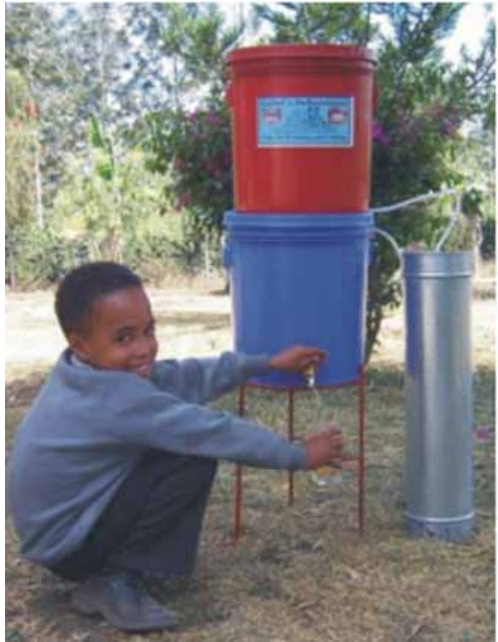
Figure 7. The domestic defluoridation filter based on bone char. 38
