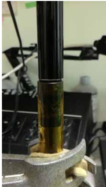
Figure 1. Electrode positions for the modified protocol, with the fluoride electrode above, and the calomel reference electrode below.
