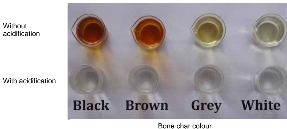
Figure 11. The standard defluoridation capacity (SDC) test without- (upper row) and with- (lower row) acidification for bone chars with different colours
